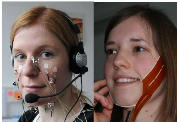
Figure 2.5: Sensor arrangement for sEMG. Source: [36]
