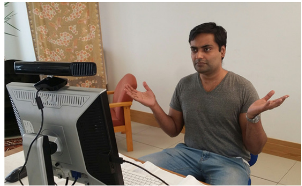
Fig. 3: Example of a gesture (“I don’t know”) which is detected by kinect in the learner state monitor module.
